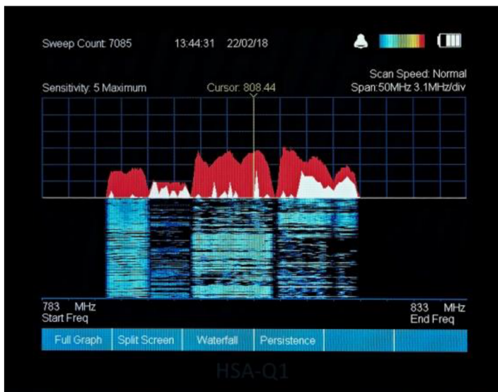
Split Screen (Half Waterfall) – Zoomed in to 50 MHz Span showing 4G Cellular Activity at 800 MHz
